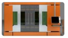
The sliding plug door design is the same as that of high-speed trains, which has high sealing performance and does not take up space.
